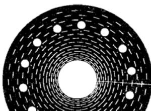
In resistive Bitter magnets, the windings are formed by perforated copper disks (see Fig. 1.2) [5,6,25] insulated from each other by mica plates. Successive copper disks slightly overlap and form a kind of spiral (a winding stairs around a central hole). The whole stack of copper and mica disks is pressed together to form a cylinder. All holes in successive disks are supposed to line up. The
